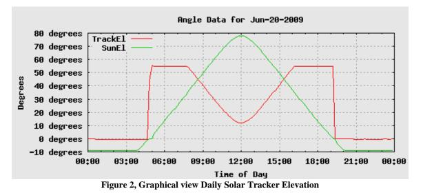
The sun's elevation is measured as 0 degrees at horizon, and 90 degrees directly overhead. The tracker's elevation is directly opposite of that. Thus a tracker's elevation of 0 degrees indicates a horizontal position, and 90 degrees would be vertical.
