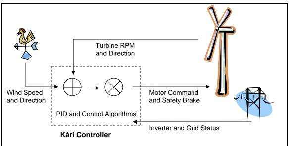
Figure 3: wind turbine control block diagram
